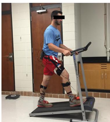
**Fig. 1.** A participant walking on the self-propelled treadmill with surface EMG sensors on the leg muscles. The walking surface is about 1.05 m in length with 15% incline.
